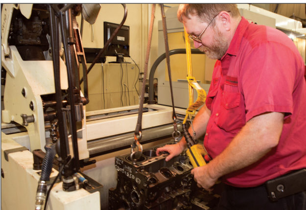
Various machining processes are used in the remanufacturing process.
