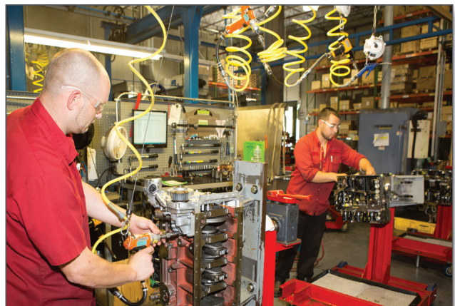
Xchange engines are built to meet original DEUTZ specifications using an assembly line process.
