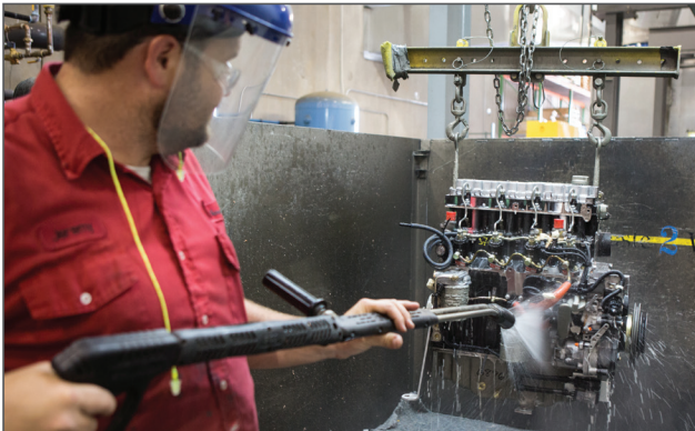
After final dress, engines are steam washed to remove any surface traces of assembly lubricant or residual testing fuel.
