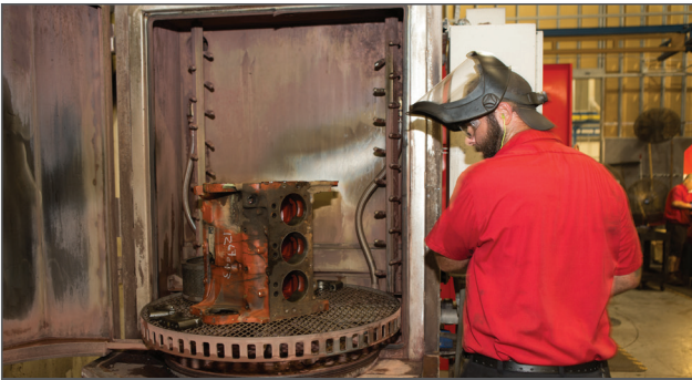
All parts receive a thorough cleaning and inspection.
