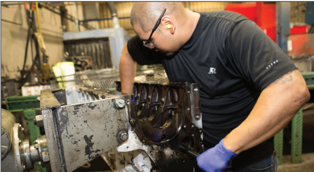
Every engine core is completely disassembled.
